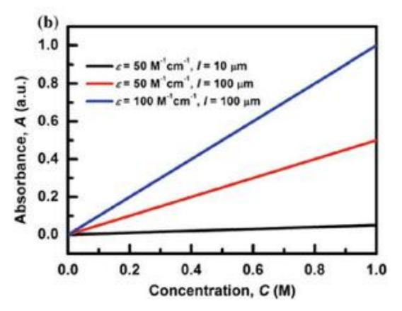
C is the concentration (M)  $\mu$  the absorptivity coefficient (M<sup>-1</sup>.m<sup>-1</sup>) l is the optical path (m)
