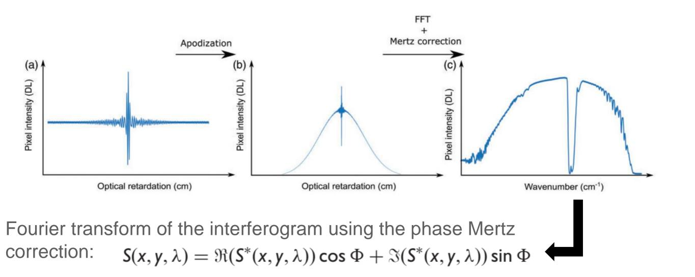
where  $S^*(x, y, \lambda)$  is the Fourier transform of  $I_a(x, y, \delta)$ , and  $\mathfrak{R}$ ,  $\mathfrak{T}$  and  $\Phi$  denote the real part, imaginary part, and phase of  $S^*$ , respectively.
