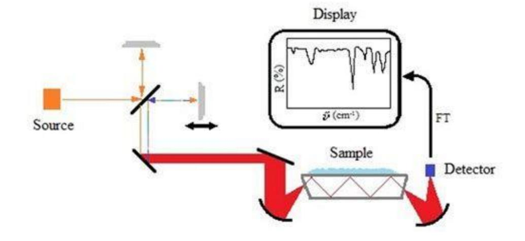
The light is reflected in a highly refracted crystal and penetrates at the surface of the sample.
