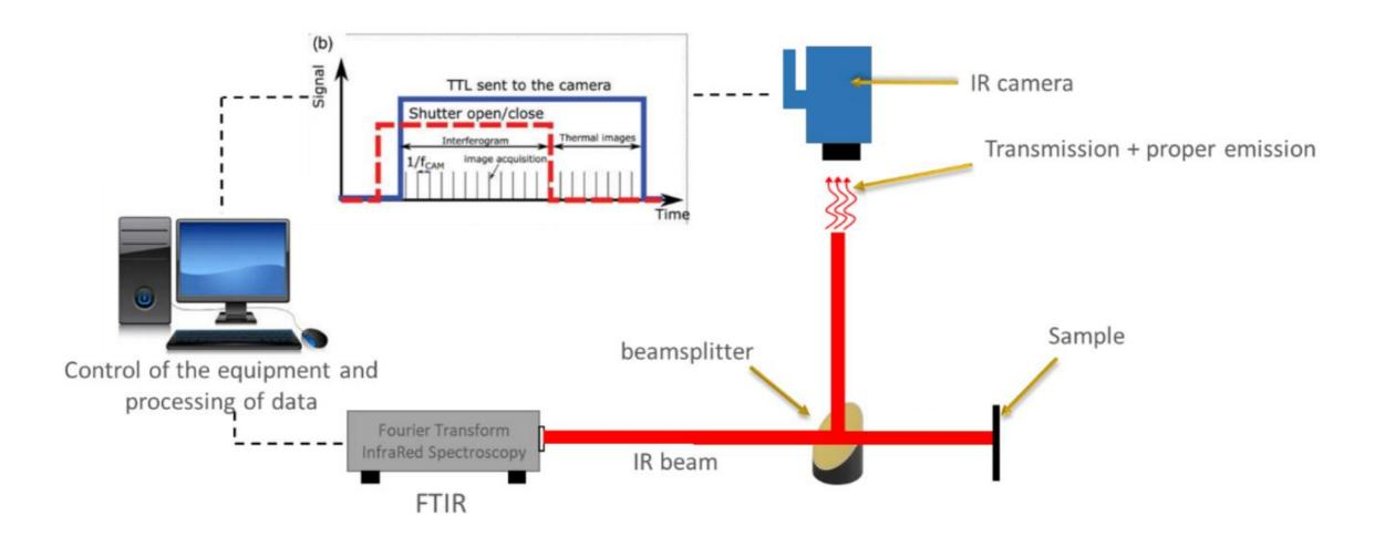
The light is reflected at the surface of the sample  $\rightarrow$  useful to capture the chemistry at surface of a solid.
