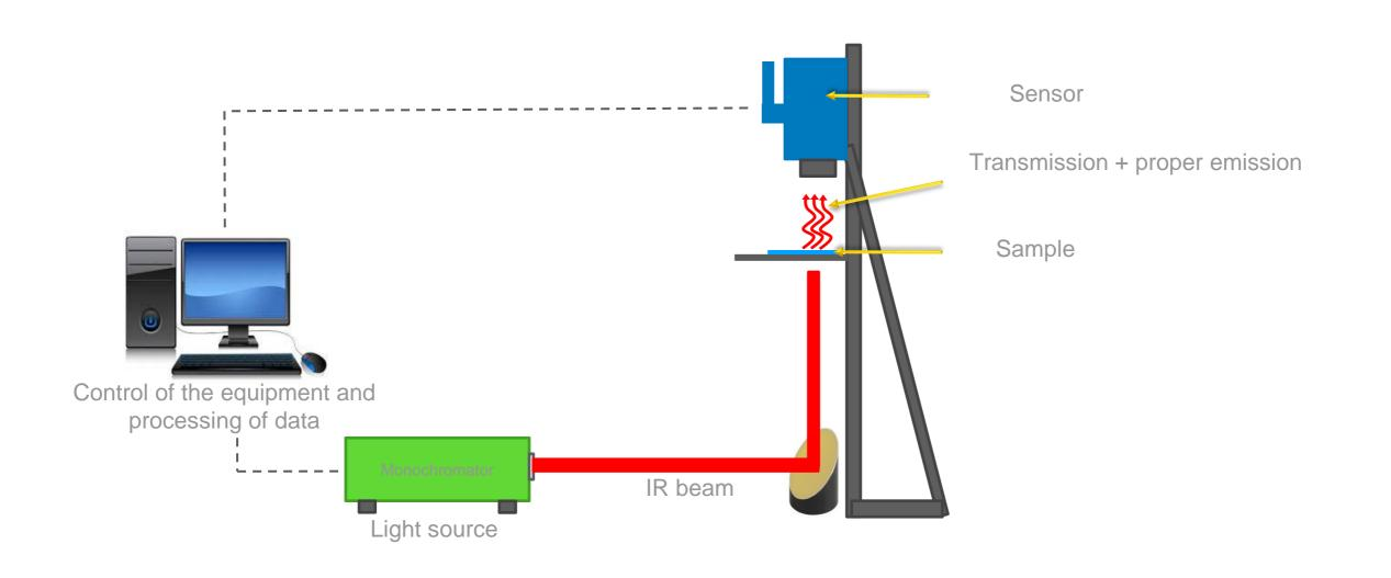
The light passes through the entire sample → more sensitive to the chemistry of sample.
