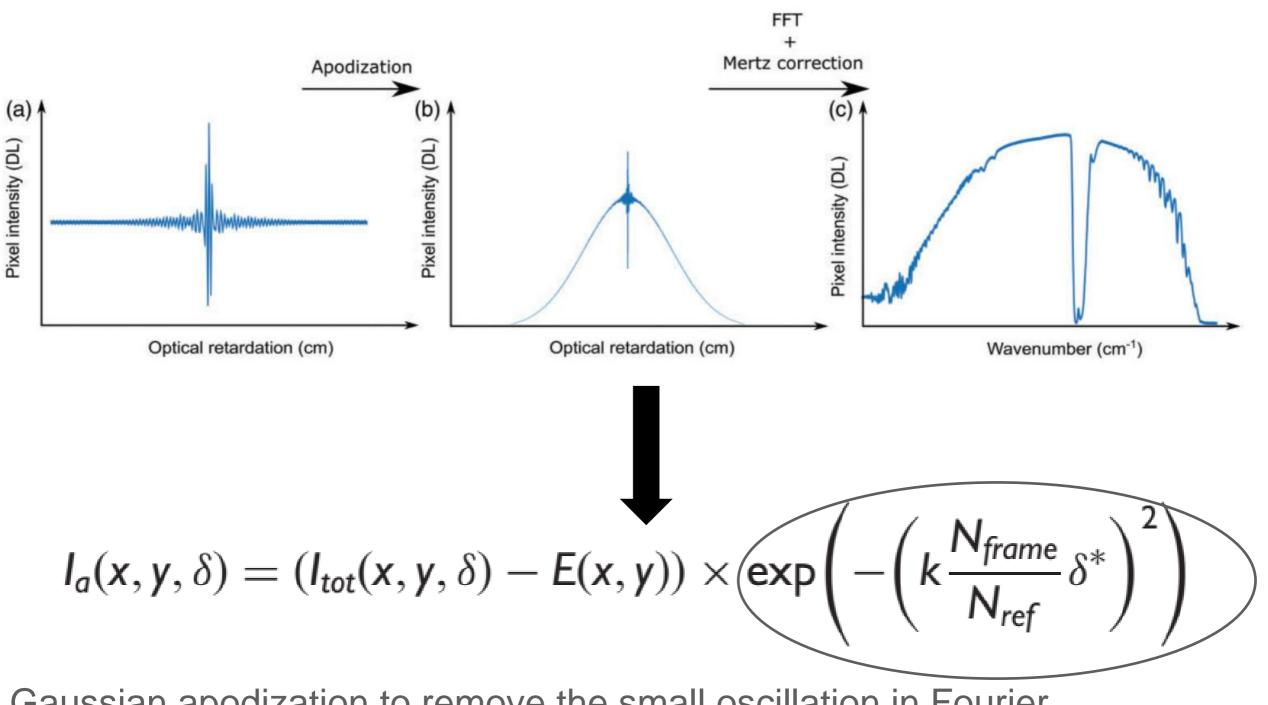
Gaussian apodization to remove the small oscillation in Fourier transformed (increase the SNR)
