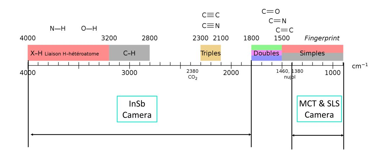
Each wavelength reveals the signature of a specific molecule or specific molecular bonding
